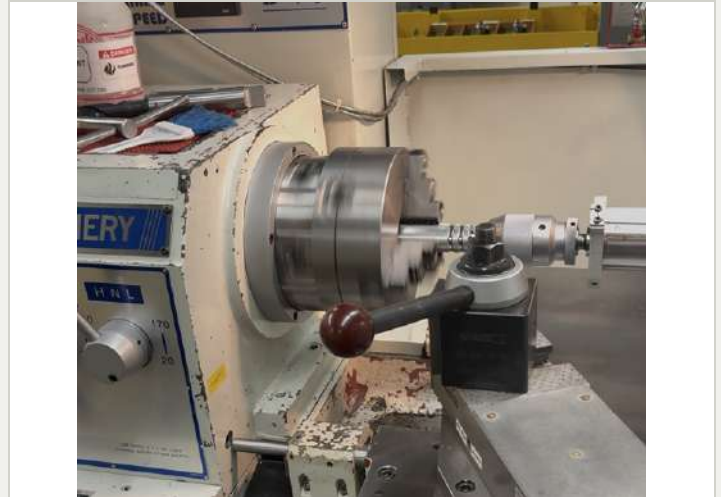
FIG 01.4 FABRICATION Lathe used to hollow each handle to 0.8125" ID for the camera + battery
