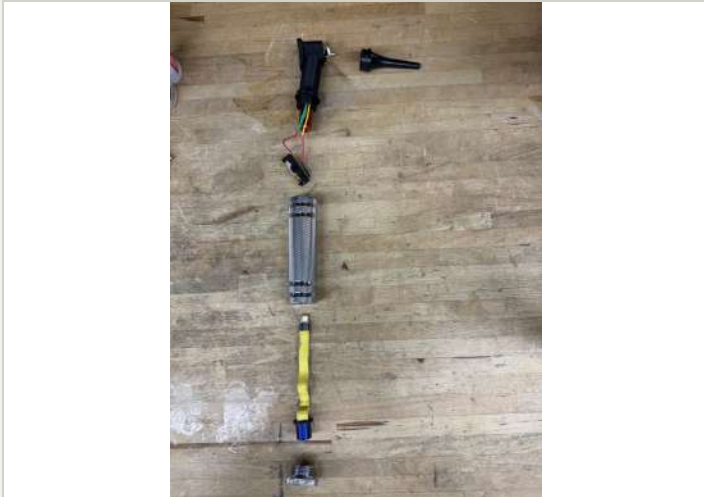
FIG 01.3 EXPLODED VIEW 3D-printed head, Bebird camera, machined knurled steel handle, rotating insert, threaded end cap
