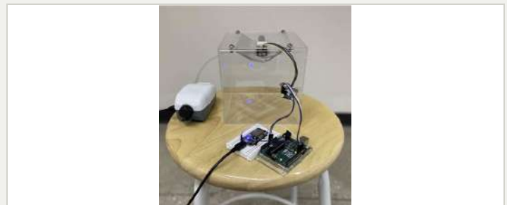
FIG 04.2 PROTOTYPE Acrylic enclosure · Arduino + WiFi alert · air pump
