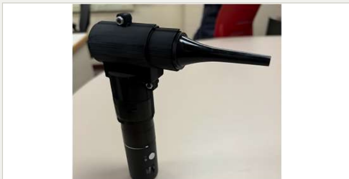
FIG 01.1 BEFORE Original BME video prototype — 0.31 lb, plastic split shell
