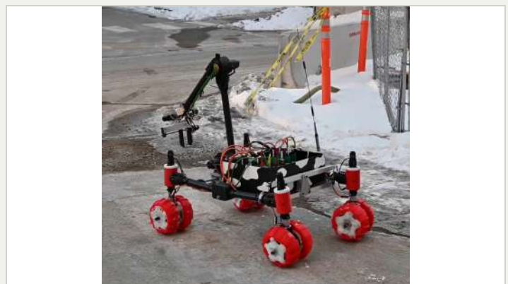
FIG 02.2 FINAL Rover with integrated swerve modules — 12th at URC
